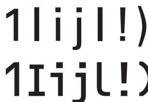
/15/ Characters that are very similar in shape get a serif, horizontal bar or curved stroke in OCR-B (bottom).
