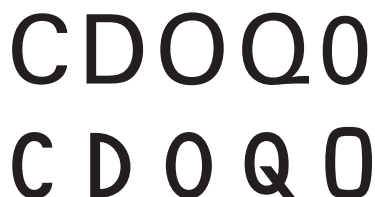
/14/ With Univers (top), the majuscules are wider and higher than the numerals; the opposite is true for OCR-B (bottom).
